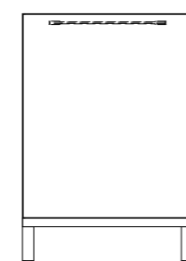
Base H723 L600 lavello e tipologia aperture Unit for sink H723 L600 and opening types
