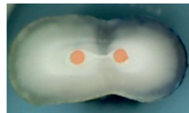
Optical microscope image of microleakage test (dye penetration test) : No dye penetration
